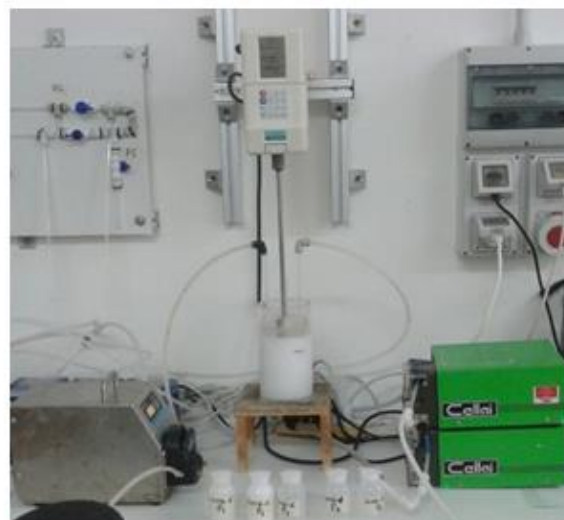
Figure 4.9: Scheme process of CSTR for the precipitation of magnesium hydroxide and calcium hydroxide from waste brine
