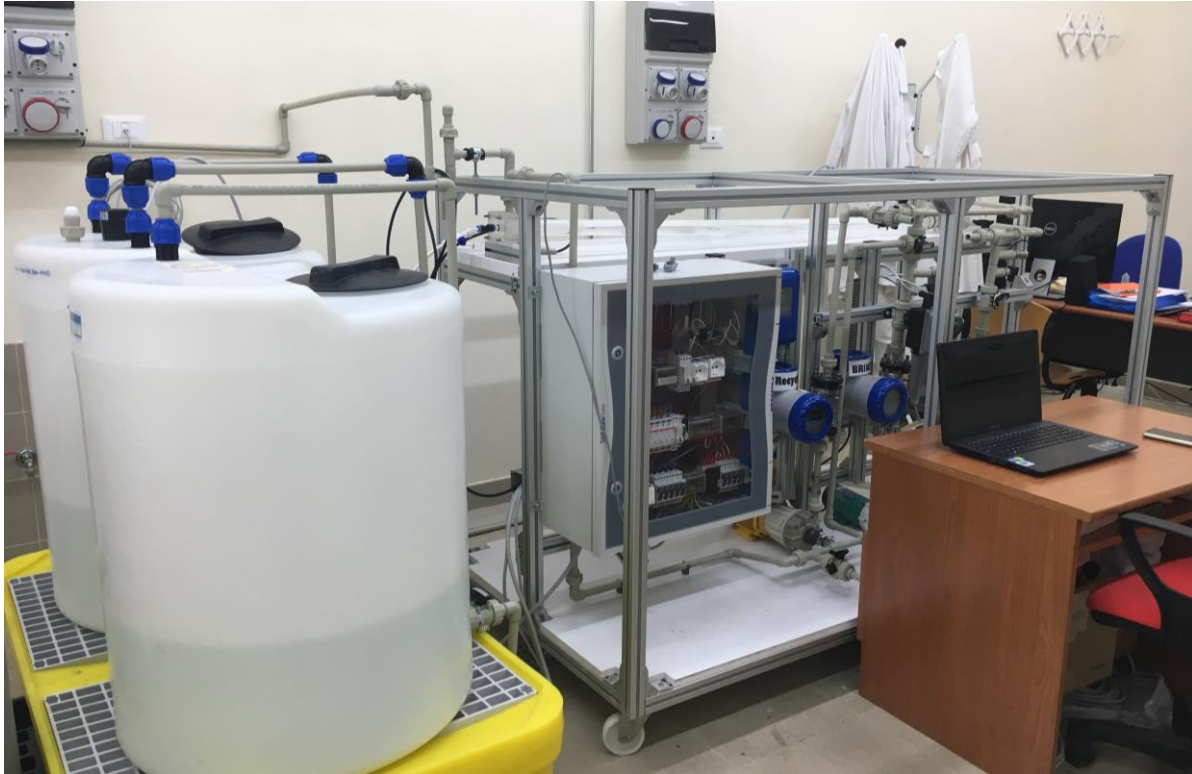
Figure 4.15: MF-PFR pilot system for the production of magnesium hydroxide and calcium hydroxide from waste industrial plant
