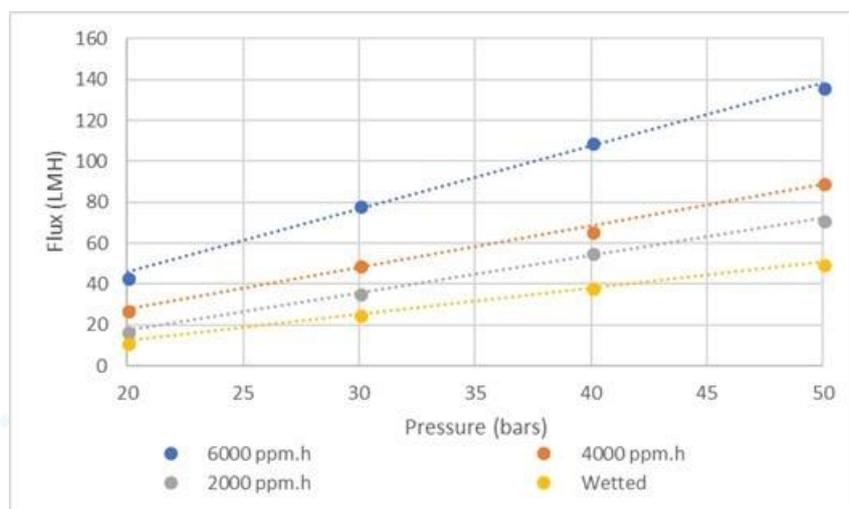
Figure 20. P vs Q curves for the SW-RO regenerated membranes at lab-scale with synthetic water.
