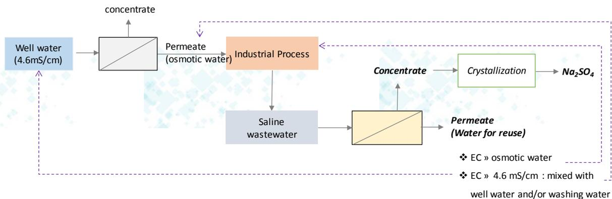
**Figure 3. Water cycle in the production process together with reuses of regenerated RO effluents.**
