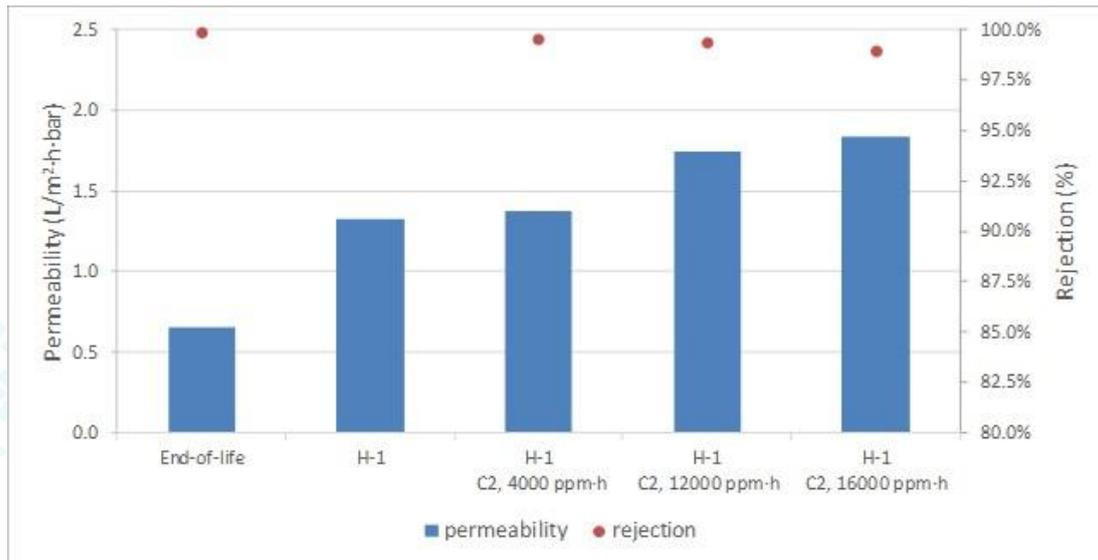
Figure 21. Effect of dose of OA on a hydrated SW-RO element. Results from NaCl standard tests.
