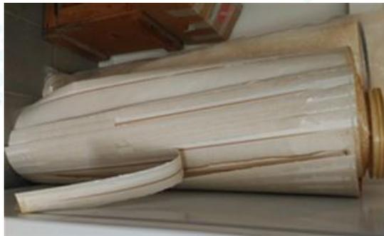
*Figure 5. BW-RO membrane element opened to access the membrane sheets.*
