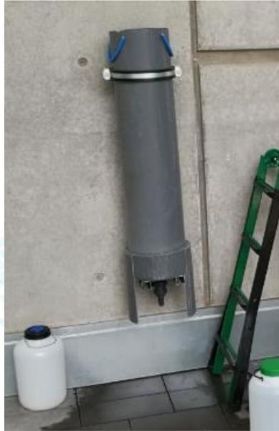
*Figure 9. PVC case for membrane elements to be hydrated.*
