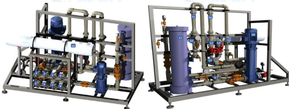
*Figure 10. 3-D model of the pilot plant used for oxidation and tests on membrane performance.*
