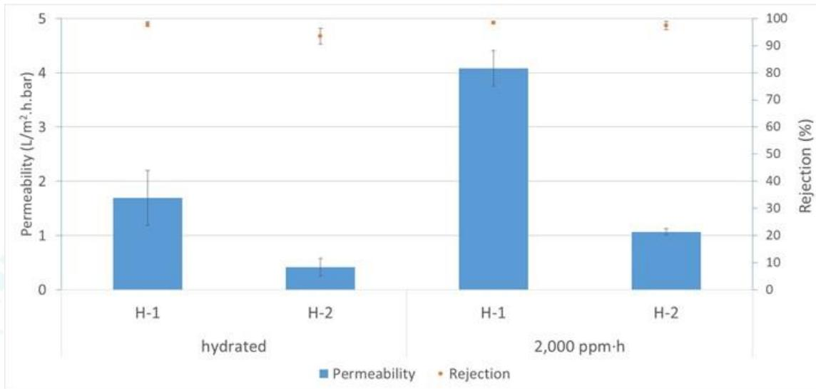
Figure 14. Effect of hydrating solvents on oxidative process of end-of-life BW-RO coupons.
