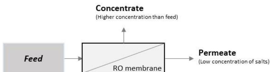
Figure 2. Effluents of a RO system.
