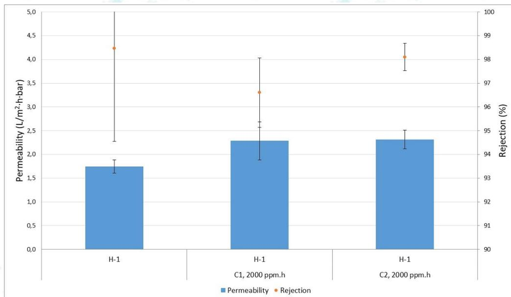
Figure 17. Effect of OA concentration on hydrated SW-RO membranes ( $n=3$ ) using a dose of  $2,000\text{ppm}\cdot\text{h}$ .
