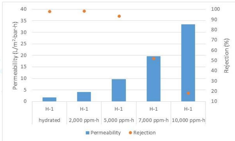
**Figure 18. Effect of OA doses on BW-RO coupons with two different hydrating solvents, H-1 (n=3).**
