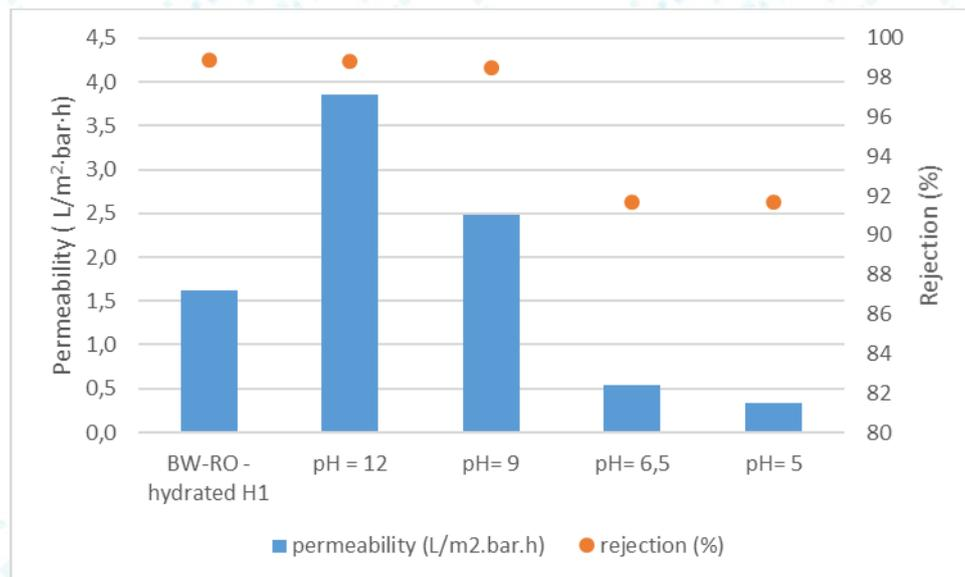
Figure 15. Effect of pH on the regeneration process of BW-RO coupons at lab-scale (n=1).
