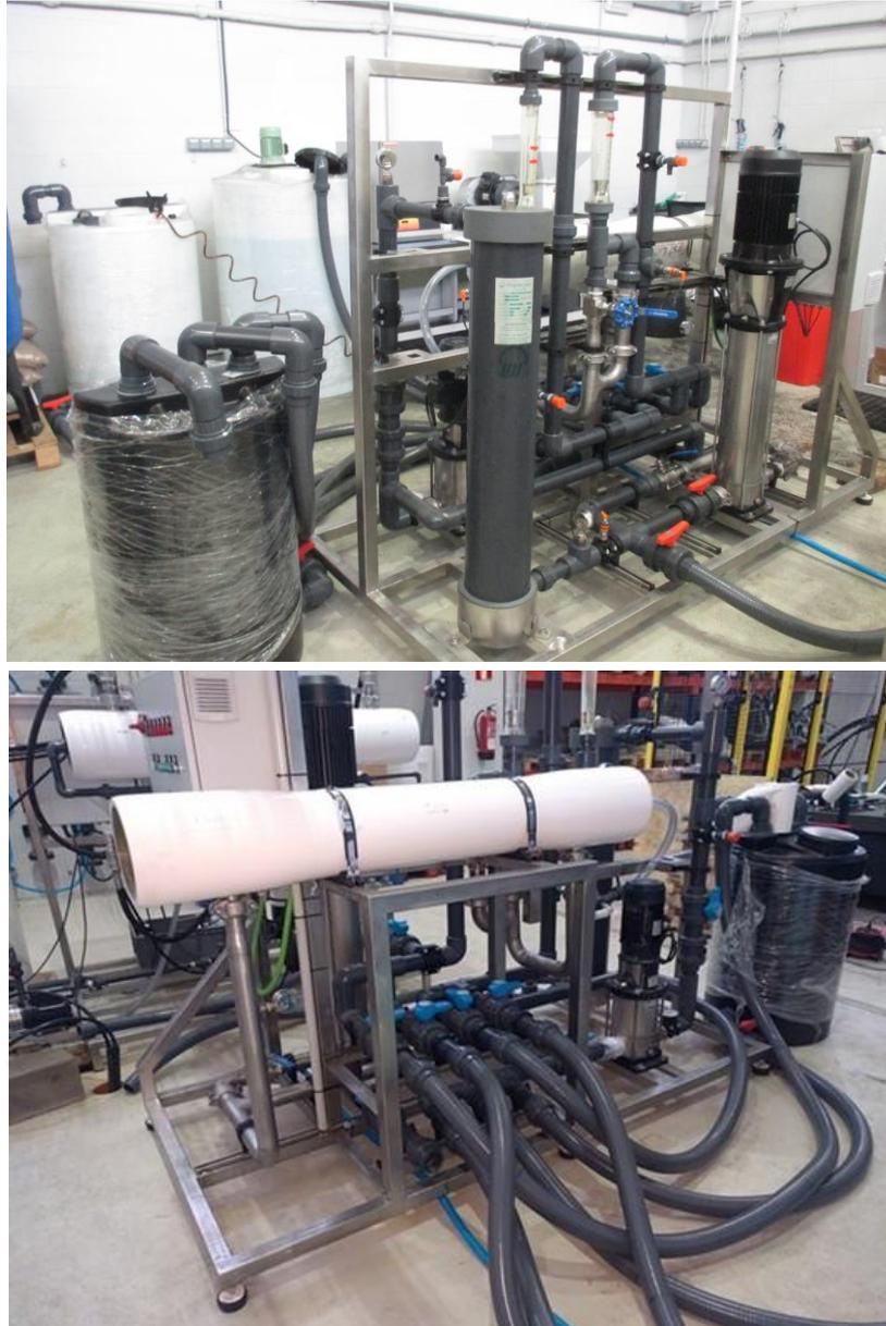
*Figure 11. Pictures of the regeneration pilot plant used for oxidation and tests on membrane performance.*
