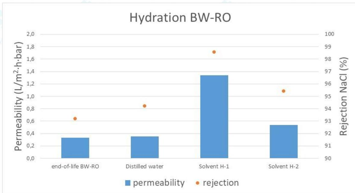
Figure 12. Effect of the hydrating solvents on end-of-life BW-RO at lab-scale (n=1).
