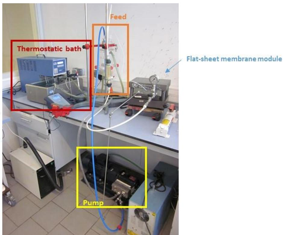
*Figure 7. Experimental set-up for membrane testing at lab-scale.*
