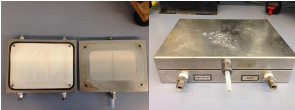
*Figure 6. Flat-sheet membrane module used for regenerated membrane tests.*
