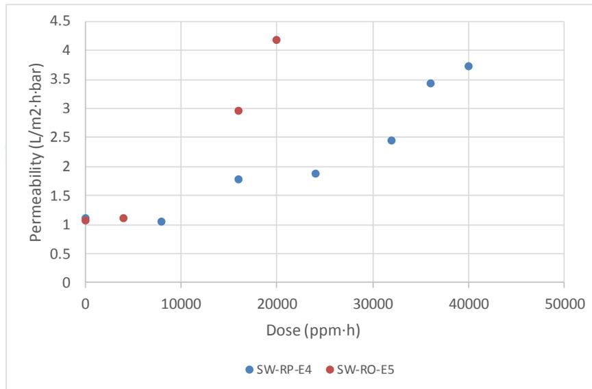
*Figure 22. Effect of the dose for the two regenerated elements*
