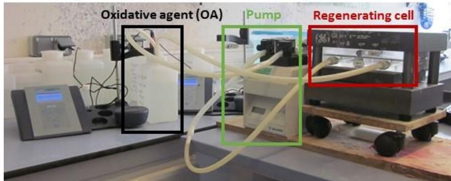
*Figure 8. Experimental set-up for oxidizing the membrane at lab-scale.*
