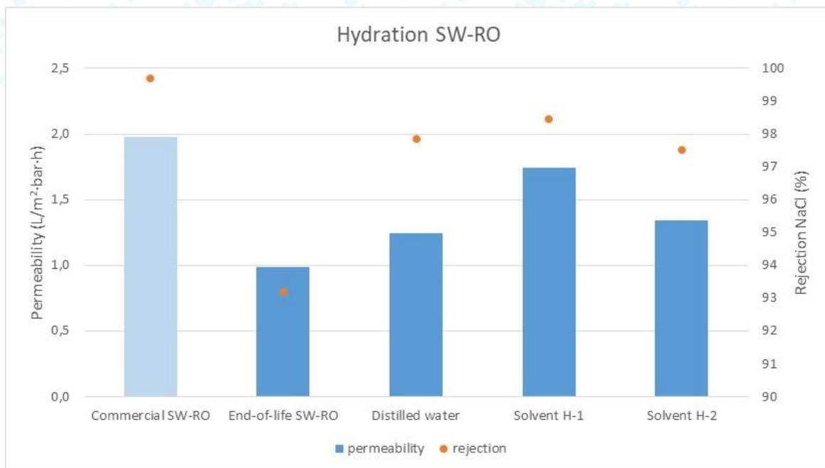
Figure 13. Effect of the hydrating solvents on end-of-life SW-RO at lab-scale ( $n=1$ ).
