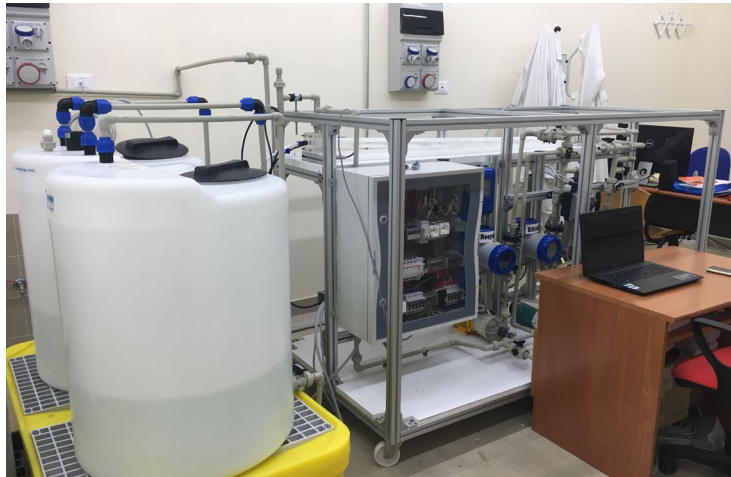
Figure 4-16: MF-PFR pilot system for the production of magnesium hydroxide and calcium hydroxide from brine
