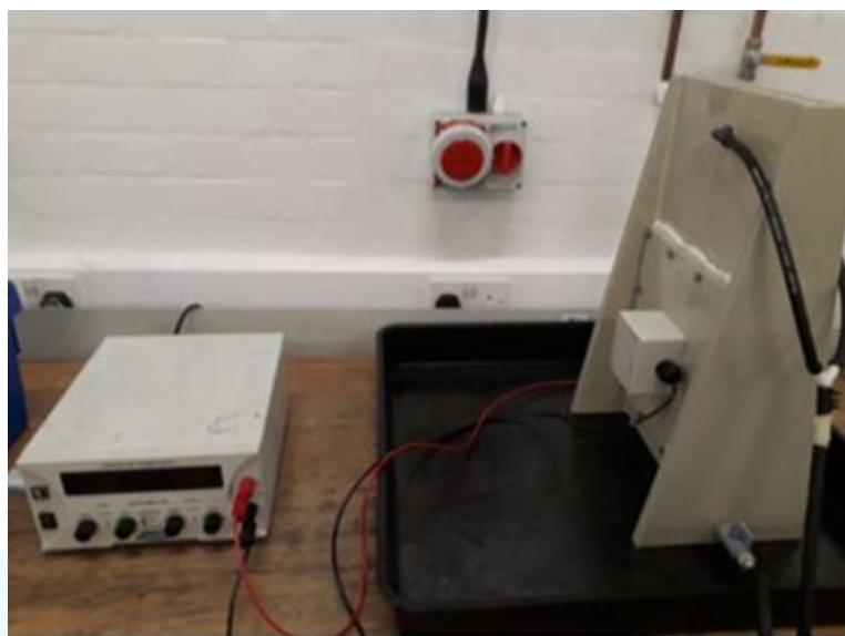
Figure 5-10: Photograph of Nyex™ 1-20e bench-scale treatment system
