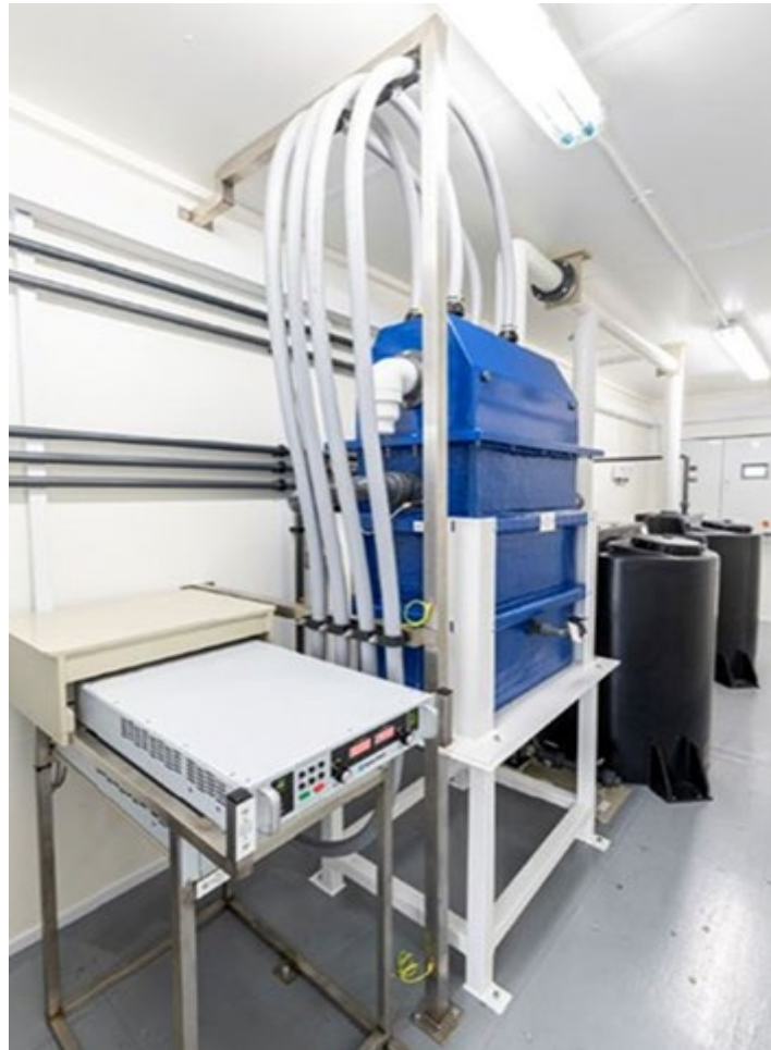
Figure 5-11: Photograph of Nyex™ 16-50e full-scale treatment system
