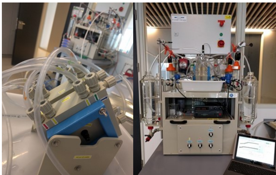
Figure 12: EDBM stack (left) and global system for the EDBM process used (right) (BP-6 from Spanish BEC).
