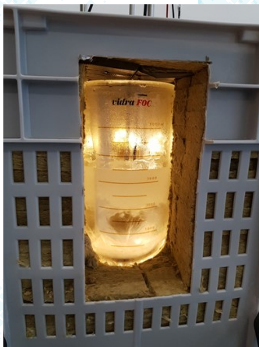
Figure 26: Scaling due to high subcooling.
