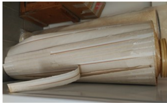
Figure 5: Membrane element opened to access the membrane sheets.
