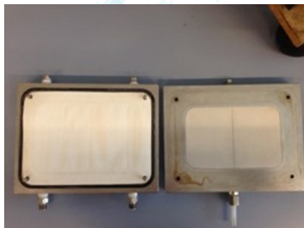
Figure 6: Flat-sheet membrane module used for regenerated membrane tests.
