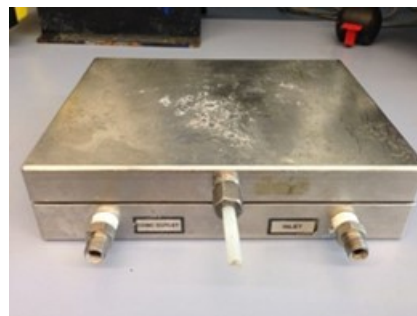
Figure 6: Flat-sheet membrane module used for regenerated membrane tests.
