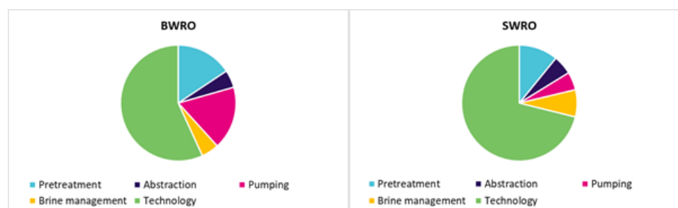
Figure 5-20. Distribution of electrical costs and requirements for BWRO and SWRO production, including brine management.
