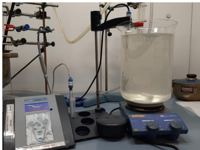
Figure 5-13. Calcium precipitation assay with 5 L of brine
