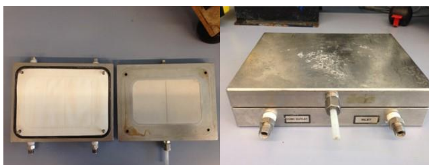
Figure 5-15. Flat-sheet testing cell used for membrane filtration assays at bench-scale
