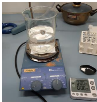
Figure 5-12. Calcium precipitation assay with 0,5 L of brine
