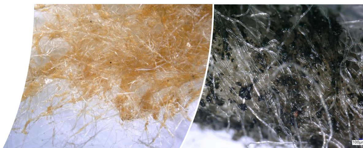
Figure 77: SEDIMENTS OF THE PIPING BEFORE THE NF FEED TANK (LEFT) AND AFTER NYEX EFFLUENT (RIGHT)
