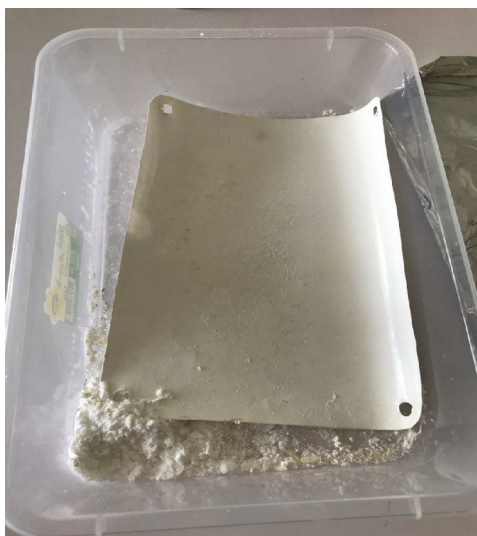
Figure 2.8 \text{Na}_2\text{SO}_4 precipitation (predominantly) on membrane surface during lab scale test
